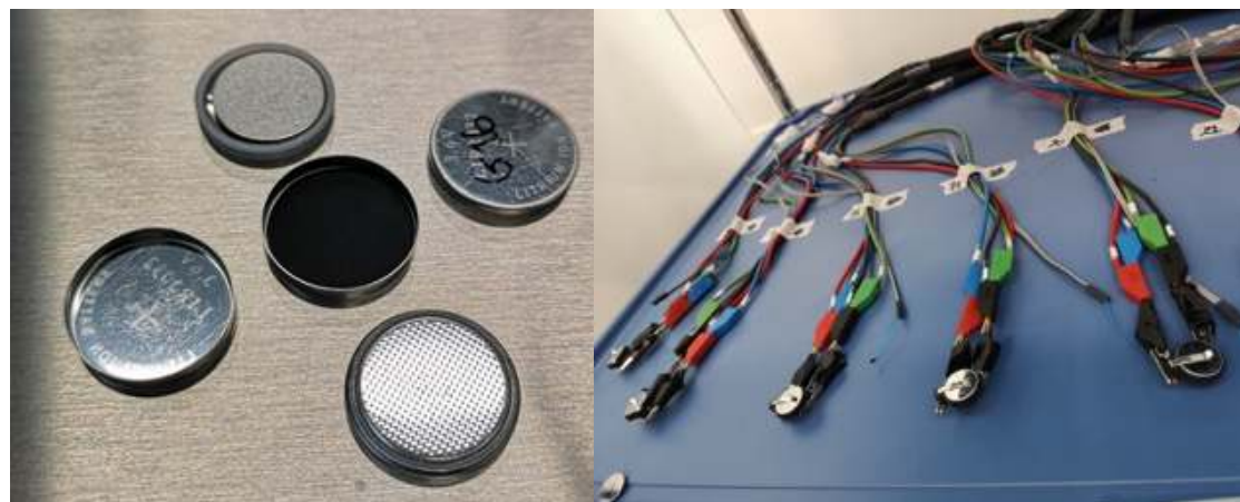
(left) Coin-cell batteries showing the graphene/composite cathode material (right) coin-cell testing at the GEIC
